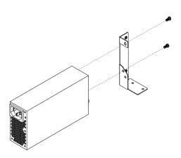
Step 2: Install the power supply to the chassis. Secure the power supply to the
