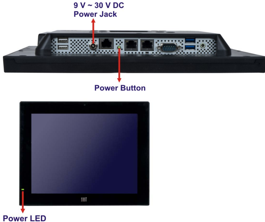
Figure 3-29: Powering On the System
