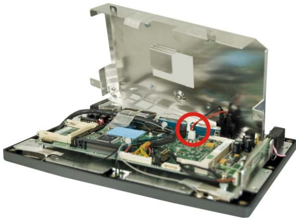
Figure 4-7: Power Switch Cable
