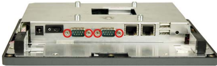
Figure 4-4: Four Hexagonal Pillars on the Bottom Panel (AFL-08AH-LX)
