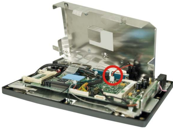
Figure 4-7: Power Switch Cable
