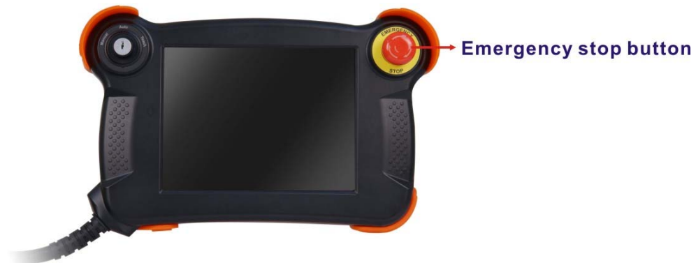
Figure 3-11: Emergency Stop Button
