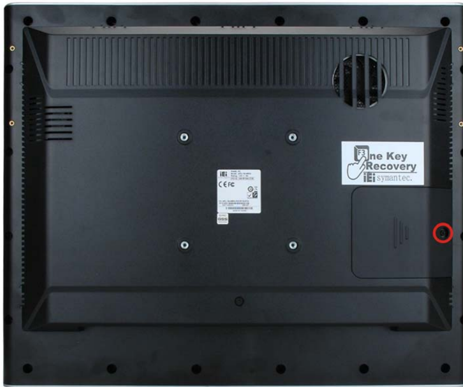
Figure 3-1: AFL-HM55 Series HDD Cover Retention Screw
