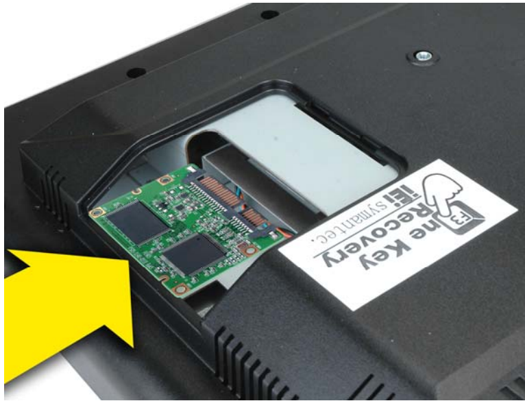
Figure 3-2: SATA DOM Card Installation
