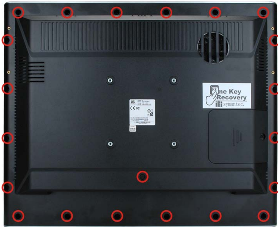
Figure 3-4: AFL-HM55 Series Back Cover Retention Screws
