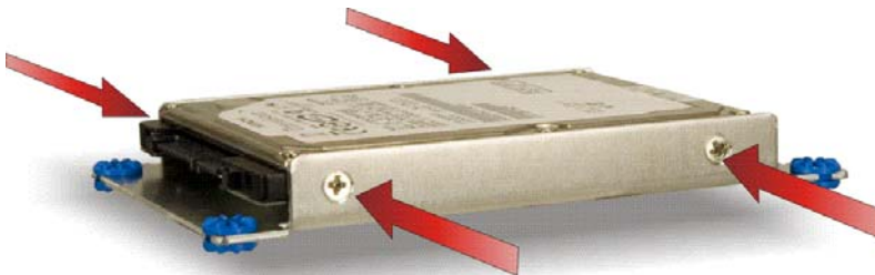
Figure 3-8: AF-12A-LX HDD Retention Screws
