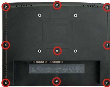
Figure 3-1: Back Cover Retention Screws
