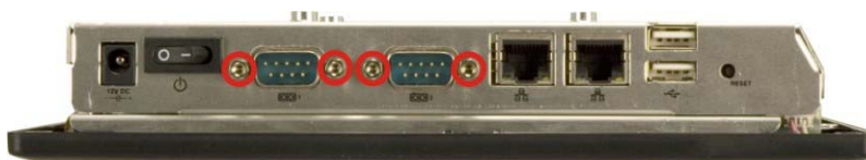
Figure 4-2: Four Hexagonal Pillars on the Bottom Panel (AFL-07A-LX)
