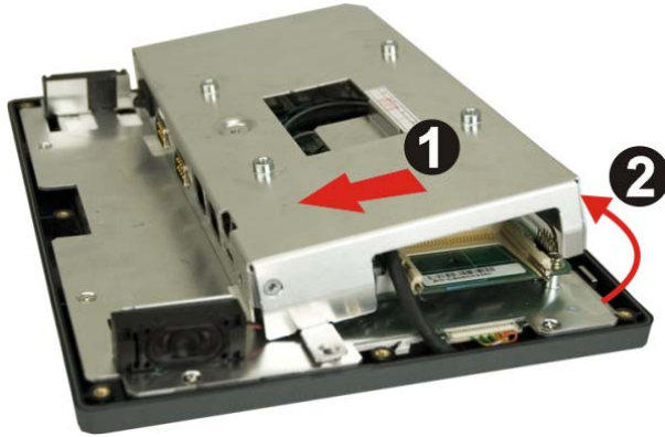
Figure 4-6: The Internal Aluminum Cover Removal
