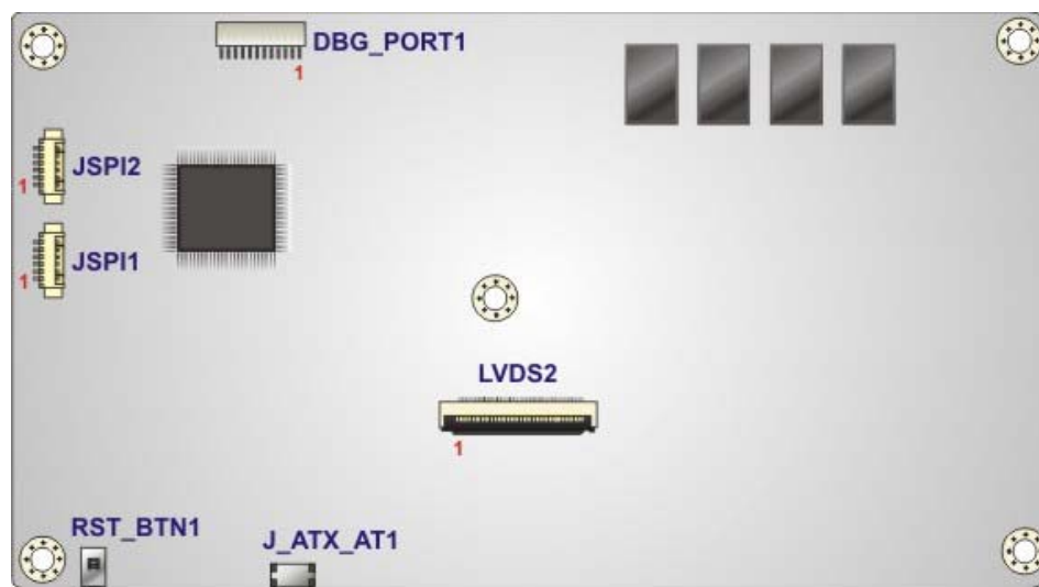
Figure 6-2: Main Board Layout Diagram (Solder Side)
