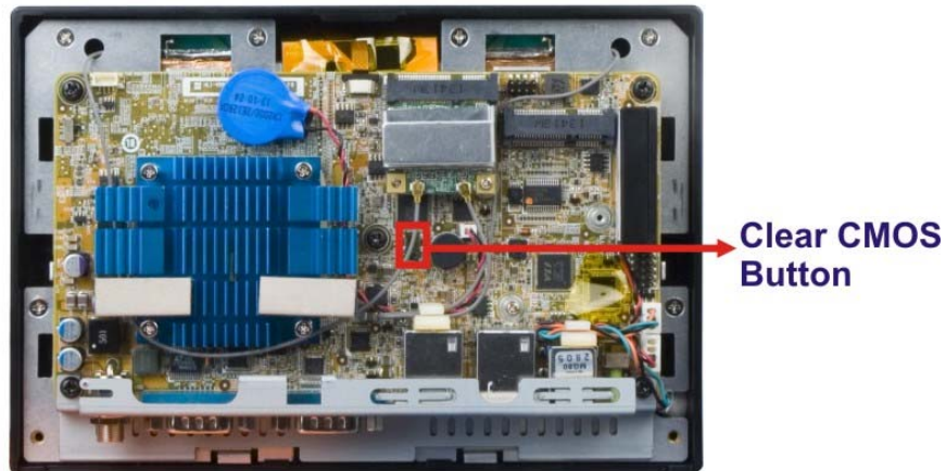
Figure 3-27: Clear CMOS Button Location
