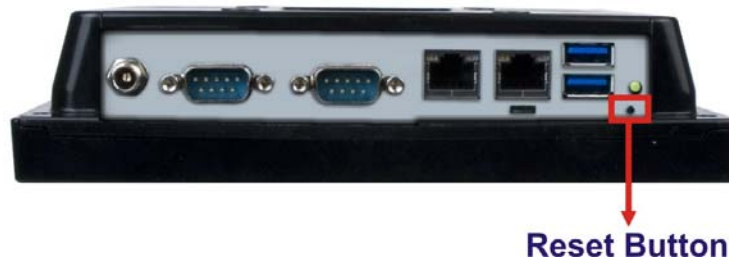
Figure 3-26: Reset Button Location
