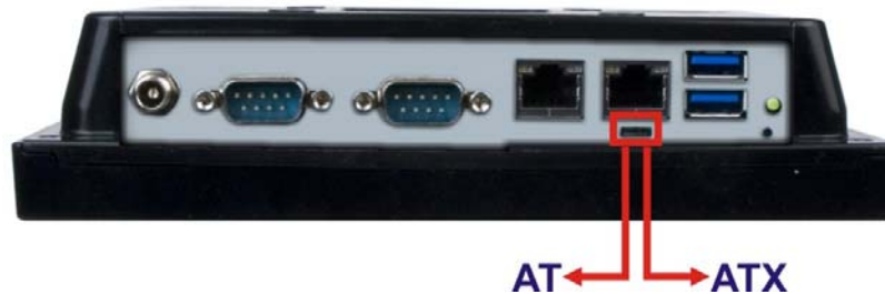
Figure 3-5: AT/ATX Switch Location
