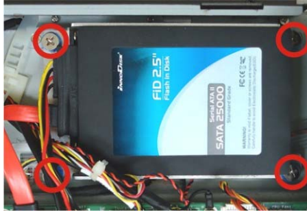
Figure 3-10: HDD Bracket Installation
