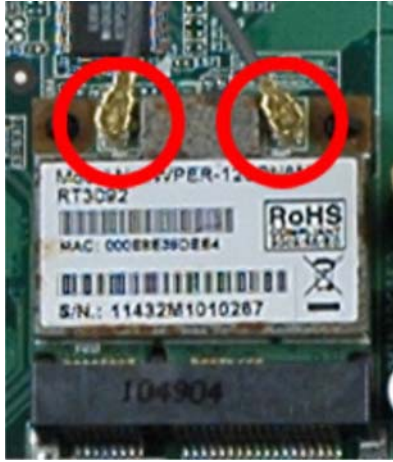
Figure 4-3: Removing the Antennas
