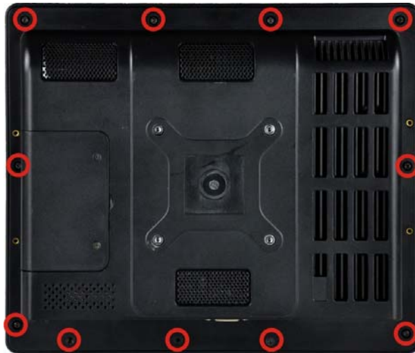
Figure 3-5: Back Cover Retention Screws
