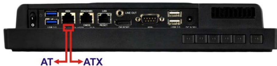
Figure 3-9: AT/ATX Switch Location
