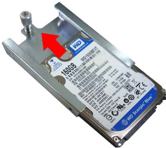
Figure 3-3: Inserting the HDD
