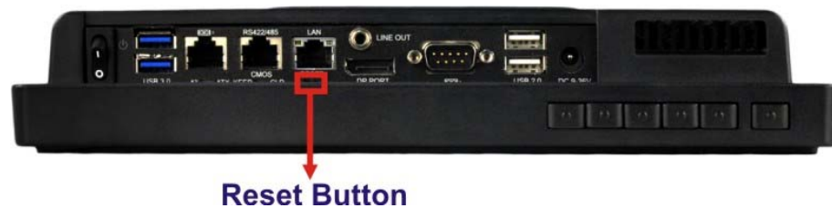
Figure 3-11: Reset Button Location
