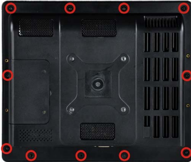
Figure 6-1: Back Cover Retention Screws
