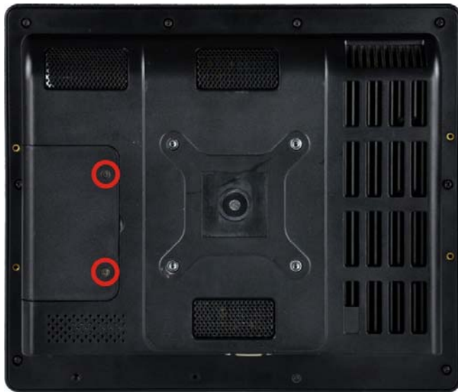
Figure 3-1: HDD Cover Retention Screws
