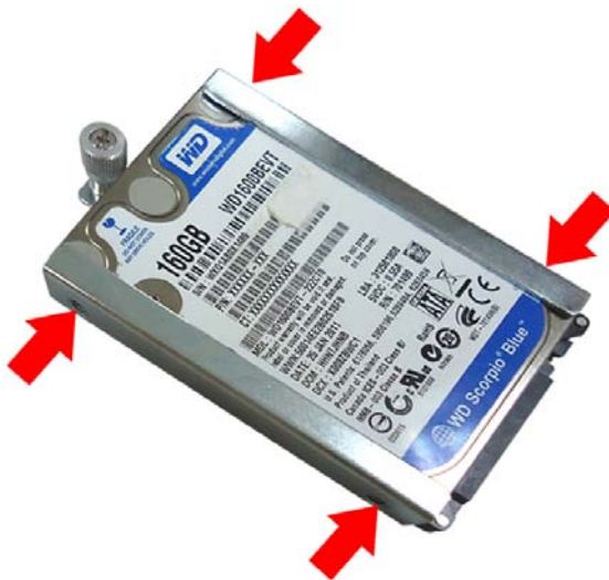
Figure 3-4: Securing the HDD
