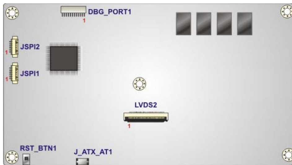
Figure 6-2: Main Board Layout Diagram (Solder Side)
