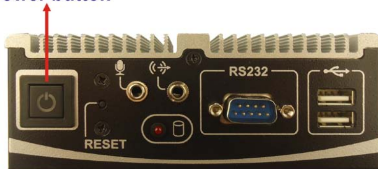
Figure 3-7: Power Button Location
