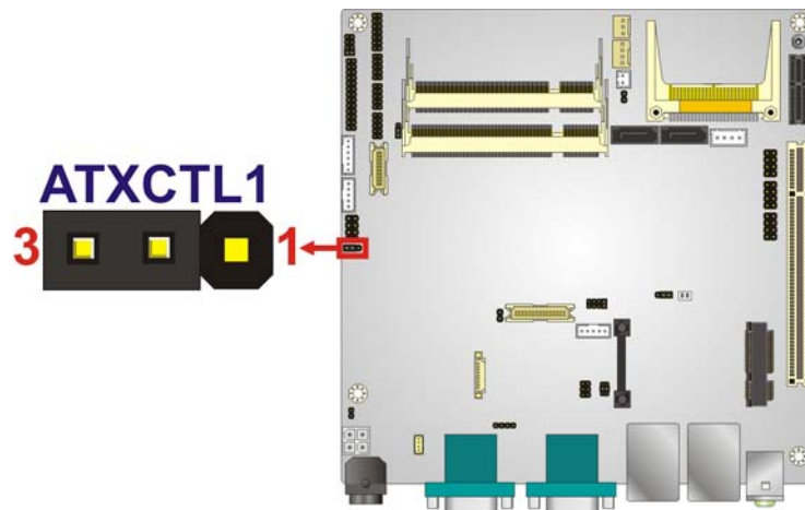
Figure 4-4: AT/ATX Power Select Jumper Location
