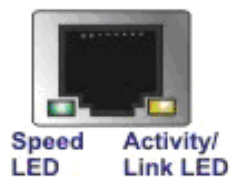
Figure 3-27: RJ-45 Ethernet Connector
