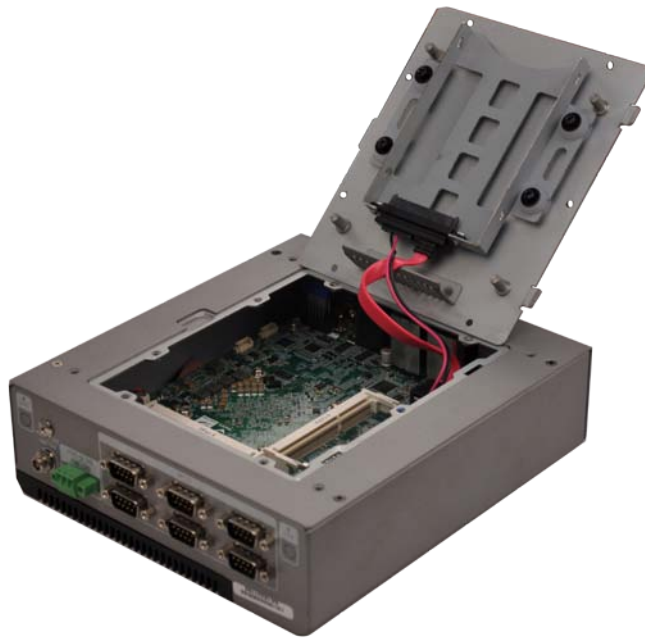
Figure 3-2: HDD Bracket Retention Screws
