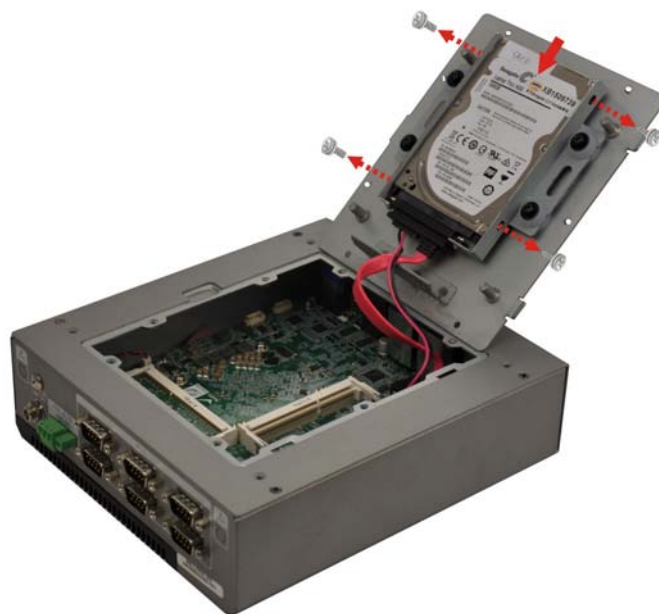
Figure 3-3: Inserting the HDD
