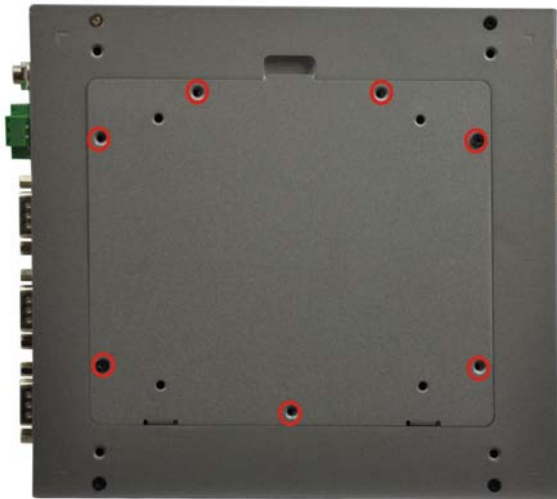
Figure 3-1: Remove Retention Screws (Bottom Panel)
