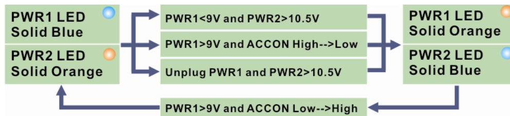
Figure 3-37: ACC On: Switch Between PWR1 and PWR2
