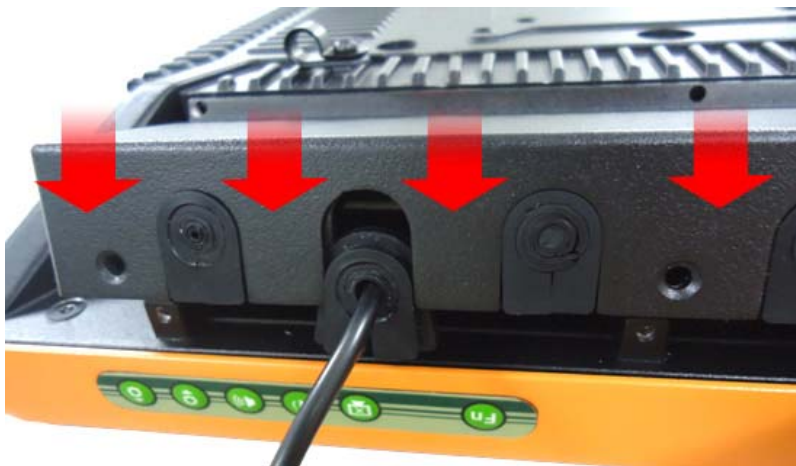
Figure 3-18: Reinstall the I/O Cover
