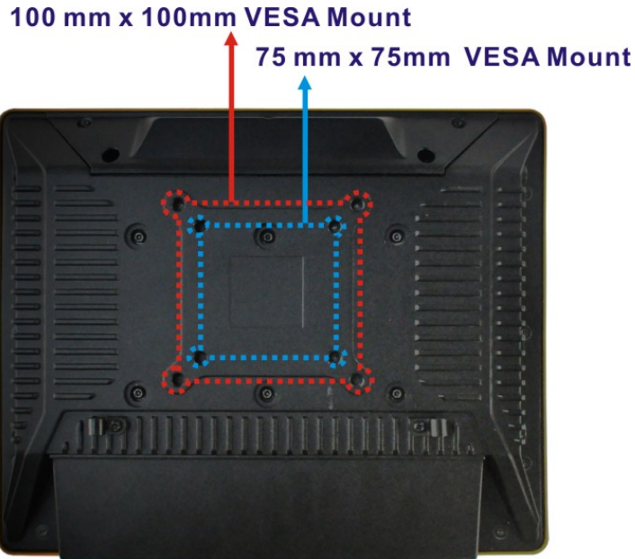
Figure 3-7: VESA Mount Retention Screw Holes
