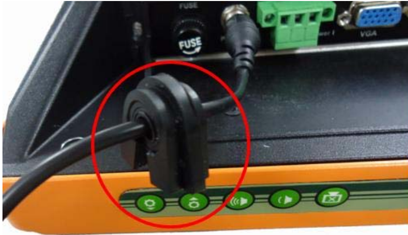
Figure 3-17: Rubber Gasket and Cable
