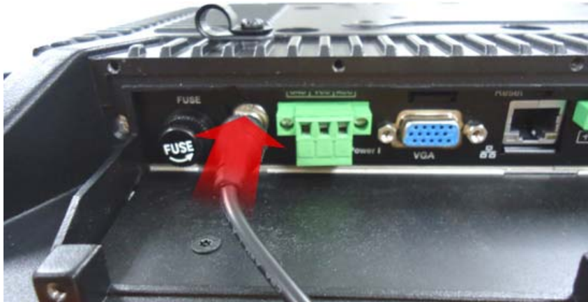
Figure 3-15: External Peripheral Device Connection
