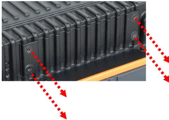
Figure 3-1: Remove the CF Card Slot Panel
