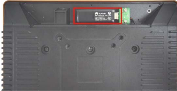
Figure 3-6: Internal USB Port Installation
