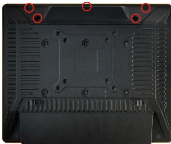
Figure 3-3: Internal USB Port Cover Retention Screws
