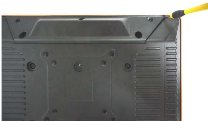
Figure 3-4: Pry along the Internal USB Port Cover
