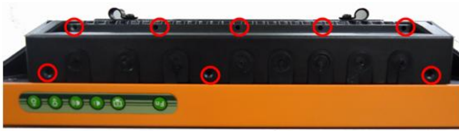
Figure 3-14: I/O Cover Retention Screws
