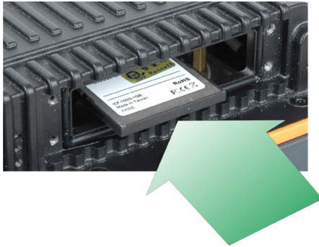
Figure 3-2: CF Card Installation
