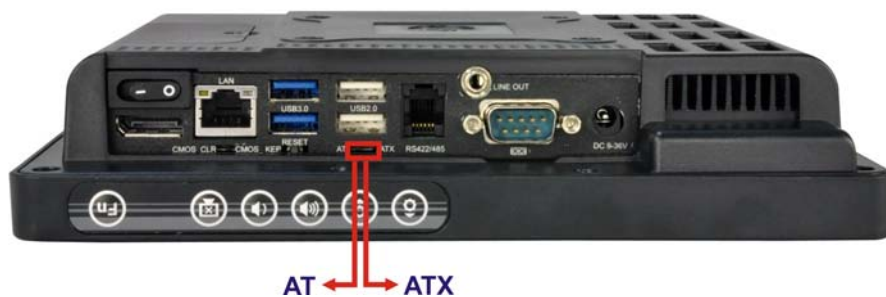
Figure 4-6: AT/ATX Switch Location
