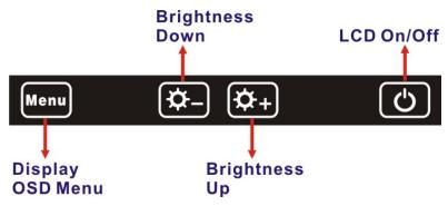
Figure 1-3: Display Control Buttons
