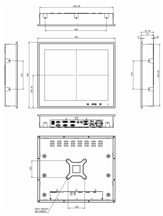
Figure 1-7: S19M Dimensions (mm)
