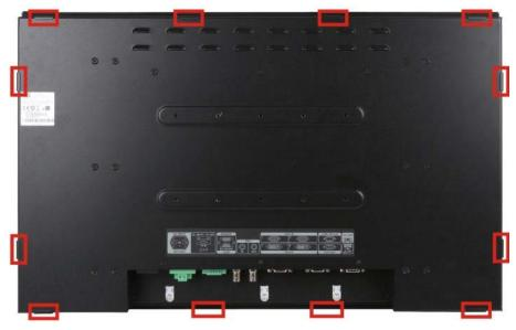
Figure 3-3: S24M Panel Mounting Hole Covers
