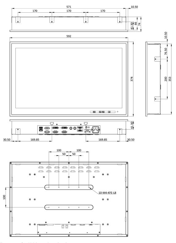
Figure 1-8: S24M Dimensions (mm)
