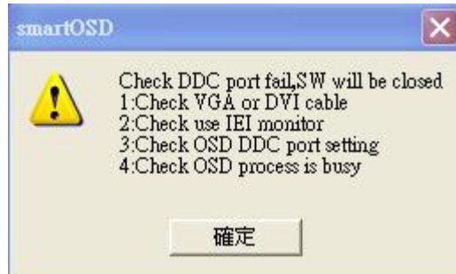
Figure C-18: DDC Port Failure
