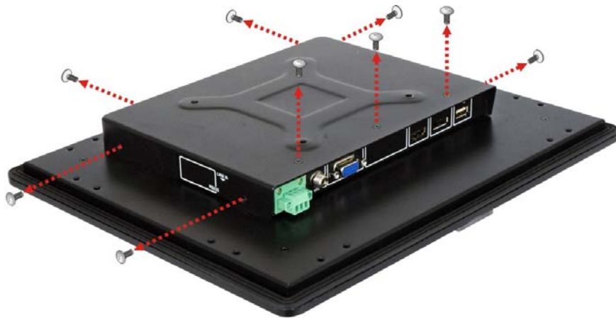
Figure 3-10: Rear Panel Retention Screw Removal (12" – 24")
