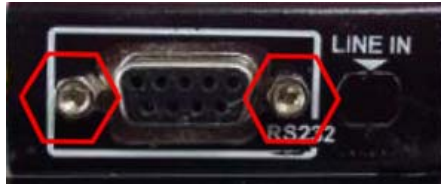
Figure 3-12: Hex Jack Screws for Securing RS-232 Connector
