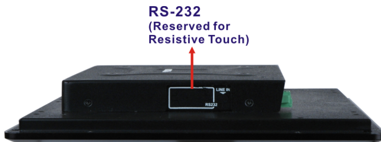
Figure 1-8: Side Panel Connector (DM-F12A/15A/17A/19A)
