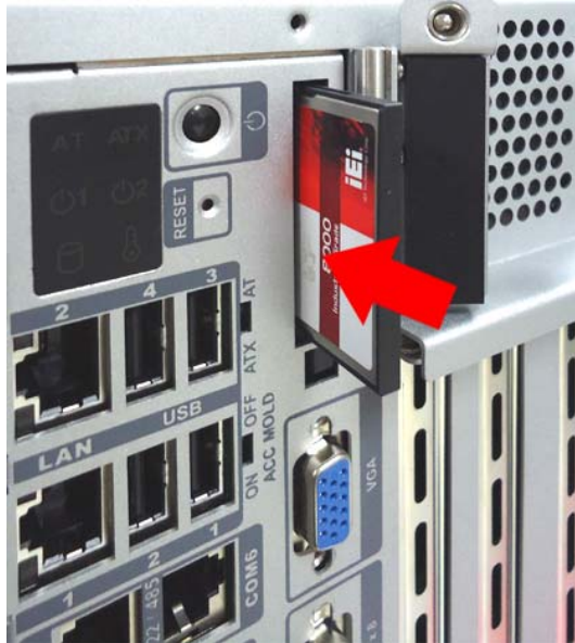
Figure 3-3: CF Card Installation
