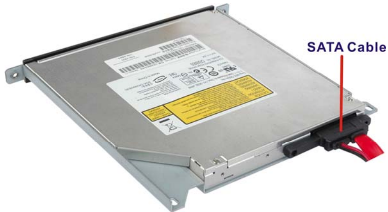
Figure 3-22: Optical Drive SATA Cable
