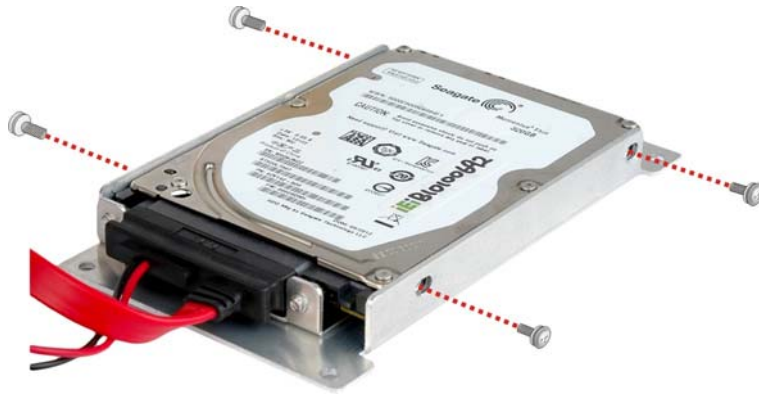
Figure 3-17: PPC-3710A-N26 HDD Retention Screws
