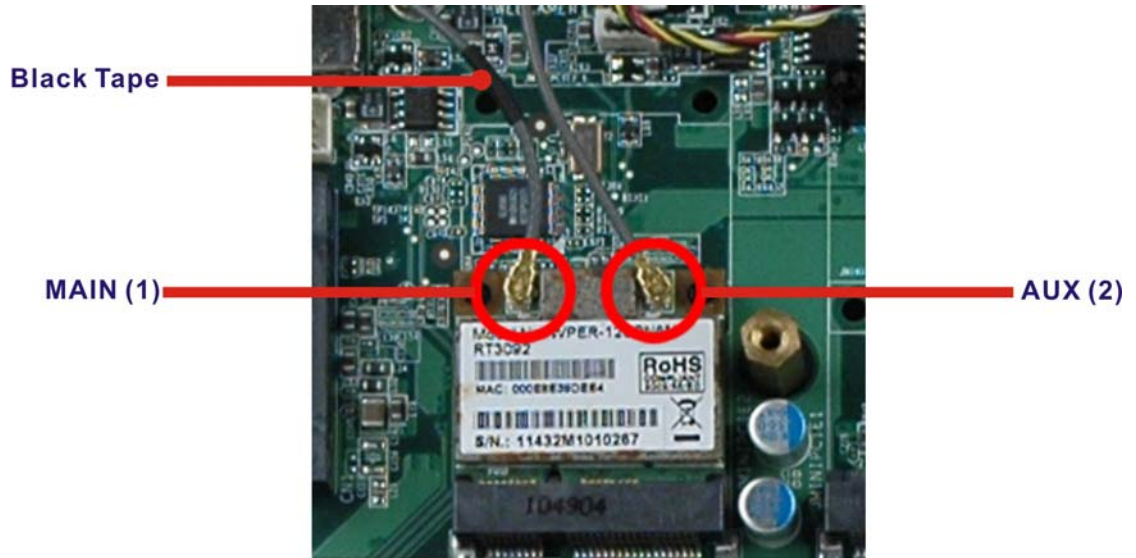
Figure 5-7: Attaching the Antennas
