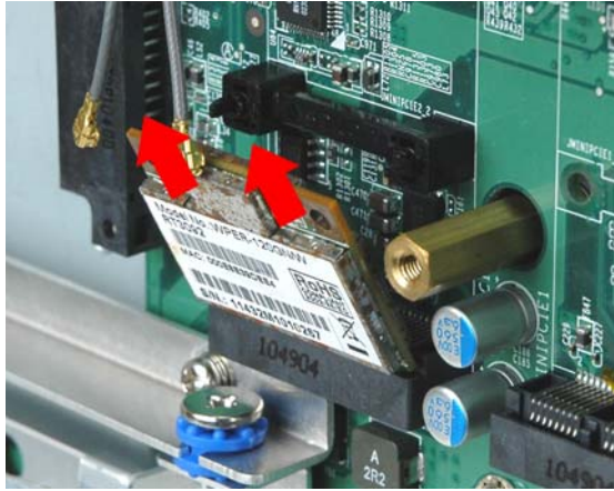
Figure 5-6: Removing the WLAN card
