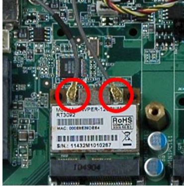
Figure 5-4: Removing the Antennas
