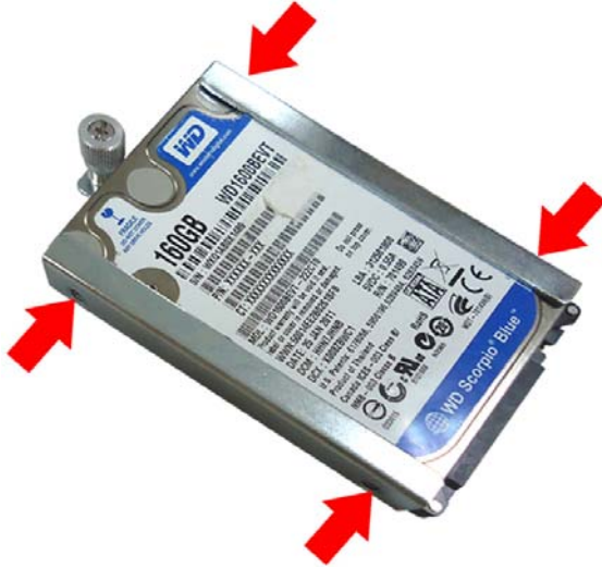
Figure 4-5: Securing the HDD
