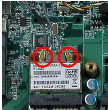
Figure 5-4: Removing the Antennas
