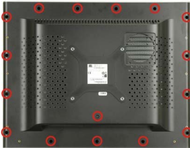
Figure 4-1: Back Cover Retention Screws
