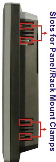
Figure 1-6: AFL-10A-N270 Side View
