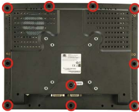
Figure 4-1: Back Cover Retention Screws
