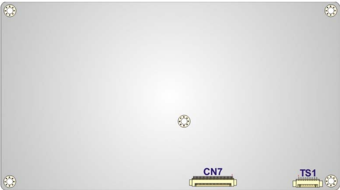
Figure 5-2: Main Board Layout Diagram (Solder Side)
