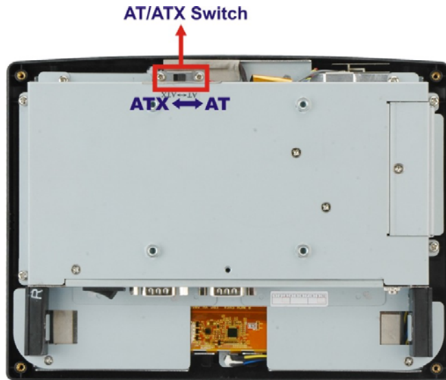
Figure 2-4: AT/ATX Switch Location
