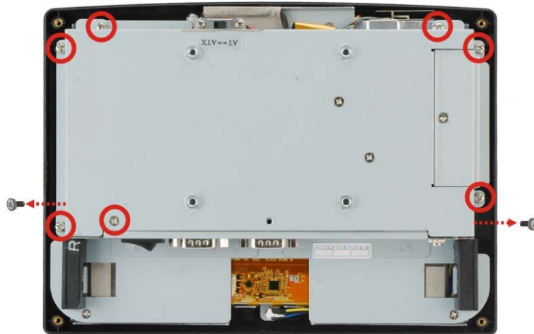
Figure 3-3: Aluminum Cover Retention Screws
