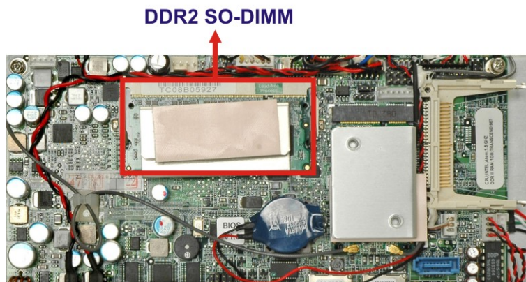
Figure 3-4: AFL-08B-N270 SO-DIMM Socket Location
