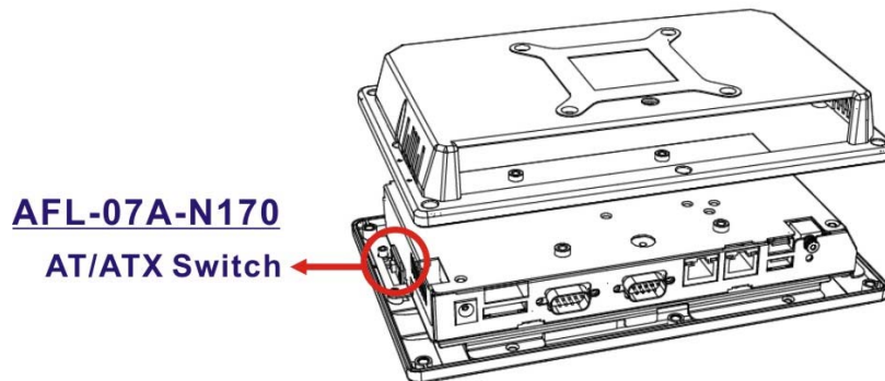
Figure 4-6: AFL-07A-N270 AT/ATX Switch Location
