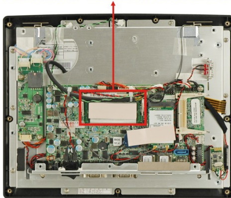
Figure 5-4: AFL-10A-N270 SO-DIMM Socket Location
