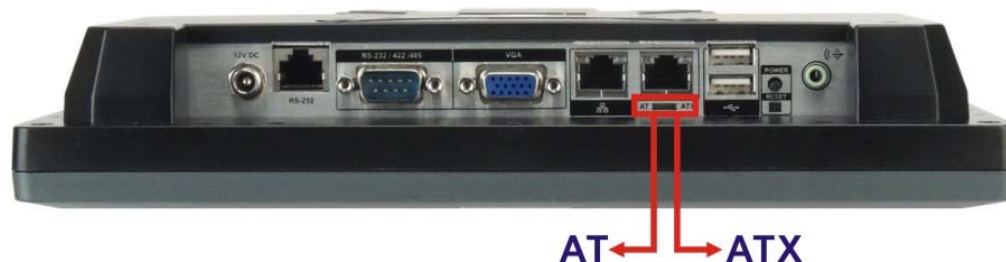
Figure 3-12: AT/ATX Switch Location
