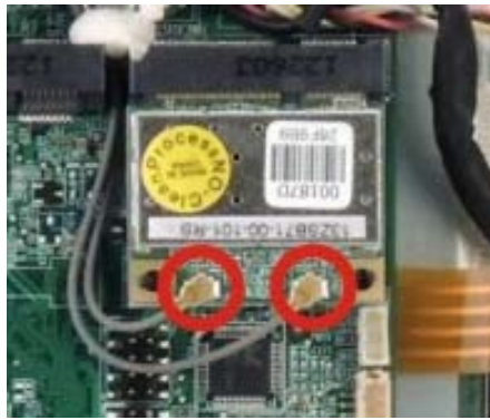
Figure 4-3: Removing the Antennas
