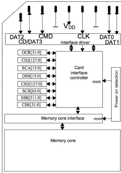
**Figure 2: Innodisk Industrial SD card 3.0 series Block Diagram**
