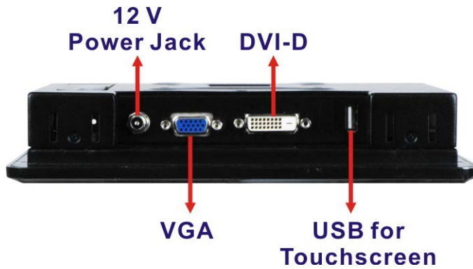
Figure 1-5: Bottom Panel Connectors (DM-F65A/08A)
