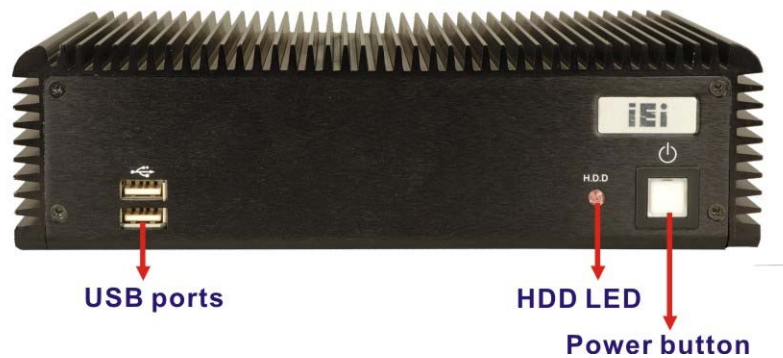
Figure 2-2: ECW-281B/B2-D525 Front Panel
