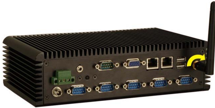
Figure 4-18: Wireless Antenna Installation
