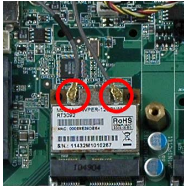
Figure 5-4: Removing the Antennas
