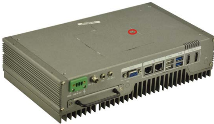
Figure 3-4: Memory Cover Retention Screw
