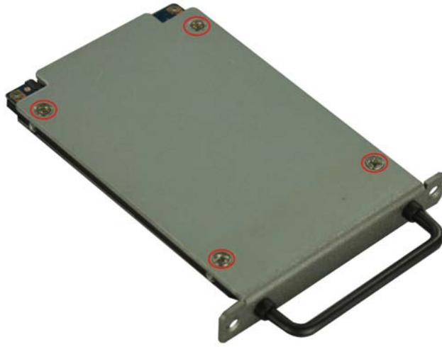
Figure 3-3: HDD Retention Screws
