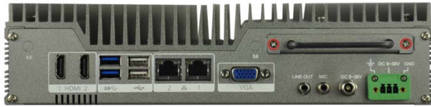
Figure 3-1: HDD Cover Retention Screws
