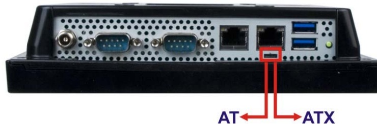
Figure 3-5: AT/ATX Switch Location
