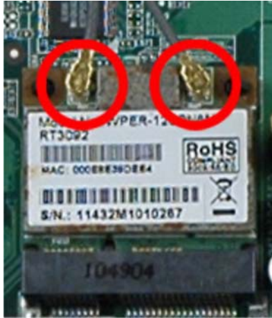
Figure 4-3: Removing the Antennas
