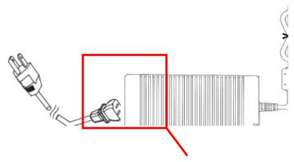
Unplug the power cord from the power adapter jack to disconnect the device.
