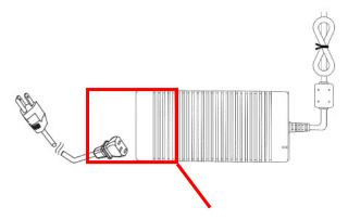
Unplug the power cord from the power adapter jack to disconnect the device.
