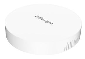
UG63 is a 8-channel lightweight indoor LoRaWAN® gateway. Adopting SX1302 LoRa chip and high-performance CPU, UG63 supports connection with more than 2000 nodes and can cover 15 km in sight and about 2 km in urbanized environment. With compact size, it is ideally suited for offices, parking lots, campuses, hotels, exhibition centers and many other indoor areas. It also applies to provide coverage for indoor blind spots.
