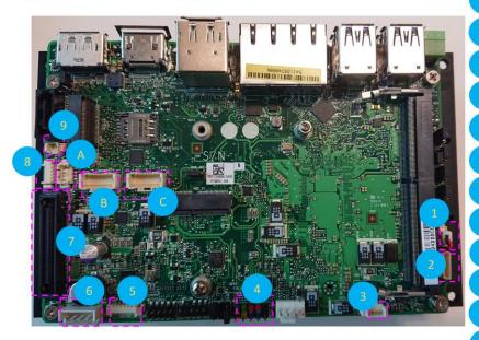
RTC Battery Socket (CR2025 cable type) Audio socket (Connect to MH-02FIO-U10) Speaker socket (Connect to 4 ohm speaker)
