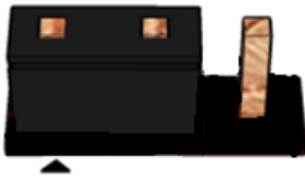
Pins 1&2: jumper position for CMOS Reset
