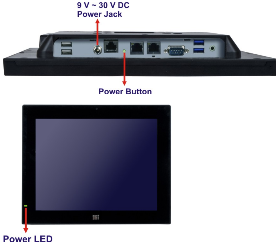
Figure 3-35: Powering On the System
