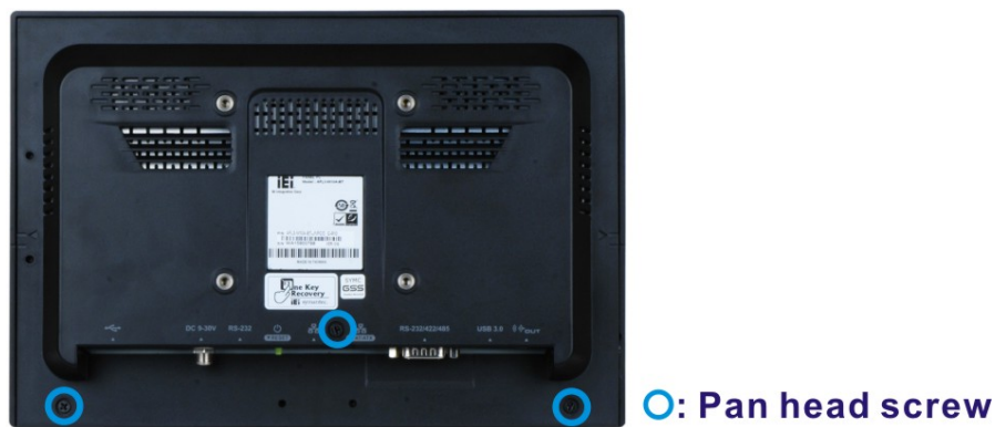
Figure 3-1: AFL3-W10A-BT Back Cover Retention Screws
