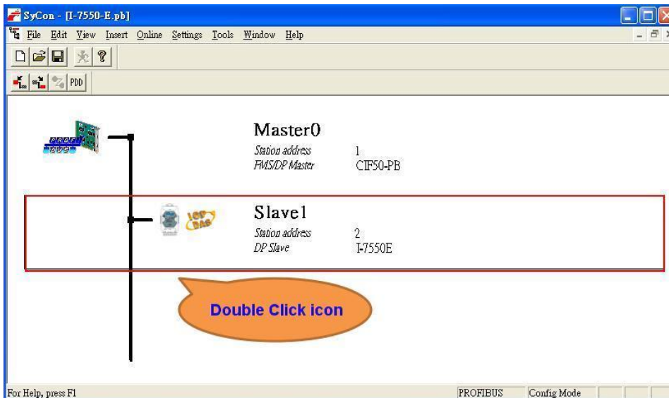
Figure 31 Double click the I-7550E icon to open the “Slave configuration” window
