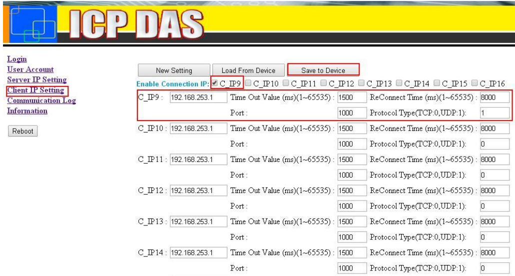
Figure 79 Set the configuration of TCP Client.
