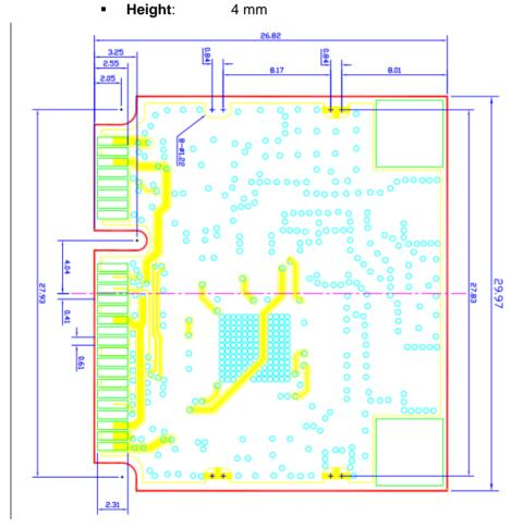
Figure 1-2: WIFI-RT3593-DB Dimensions (mm)
