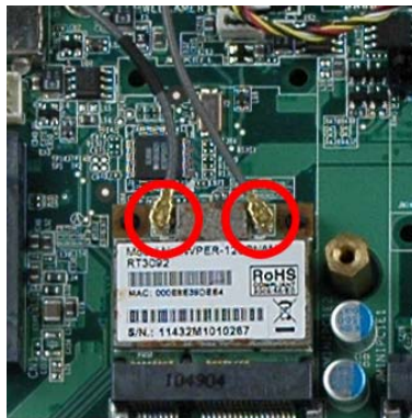
Figure 7-5: Removing the Antennas
