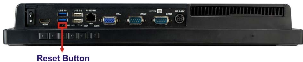
Figure 3-13: Reset Button Location
