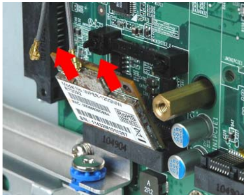
Figure 7-7: Removing the WLAN card
