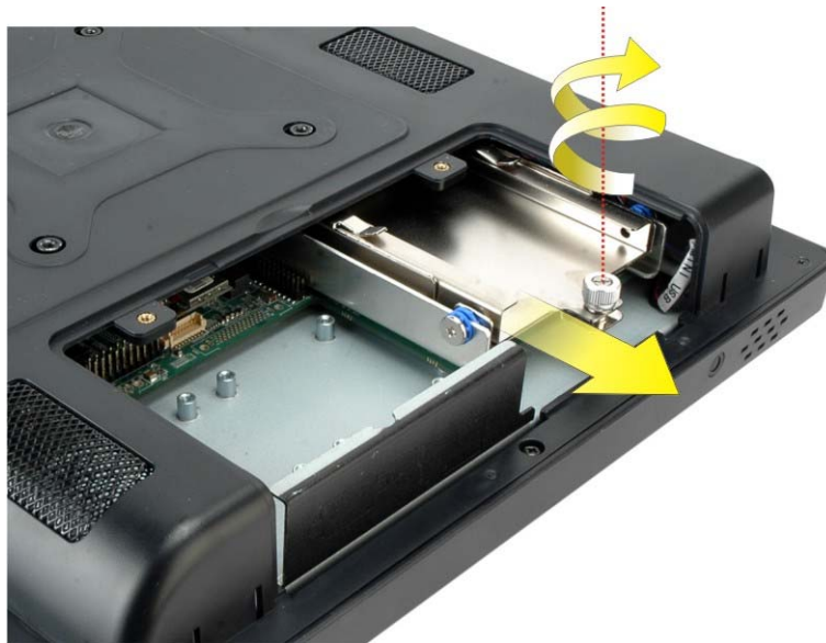
Figure 3-2: HDD Bracket Removal
