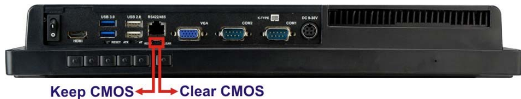
Figure 3-12: Clear CMOS Switch Location
