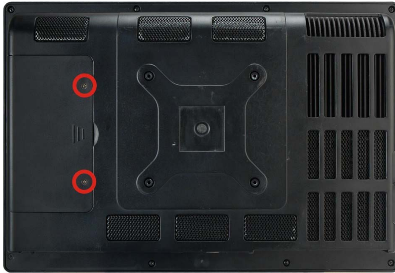
Figure 3-1: HDD Cover Retention Screws
