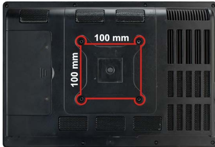
Figure 3-22: Arm Mounting Retention Screw Holes
