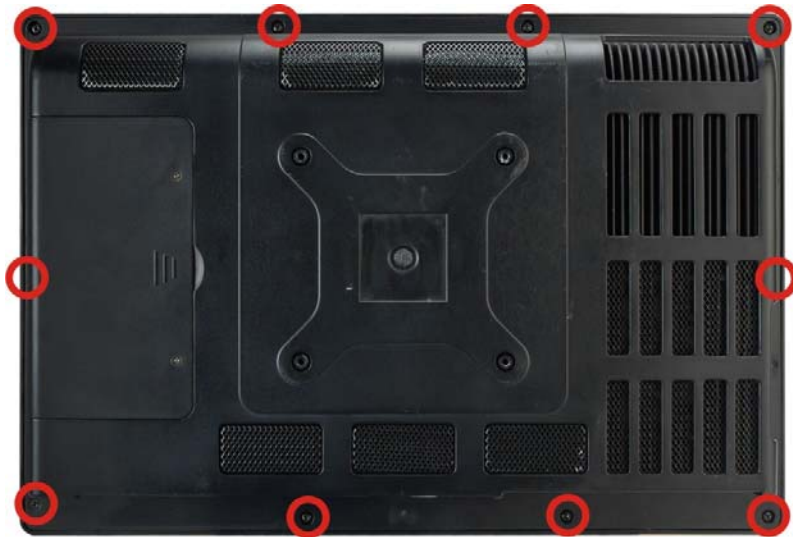
Figure 3-7: Back Cover Retention Screws
