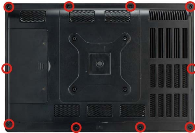
Figure 7-1: Back Cover Retention Screws
