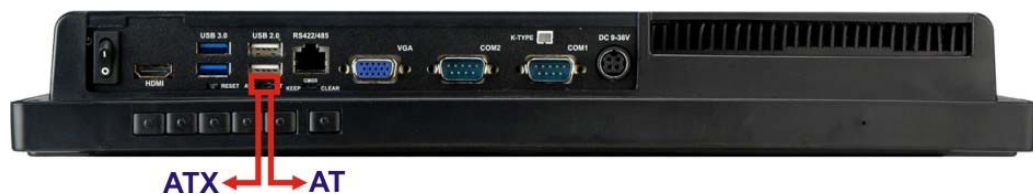
Figure 3-11: AT/ATX Switch Location
