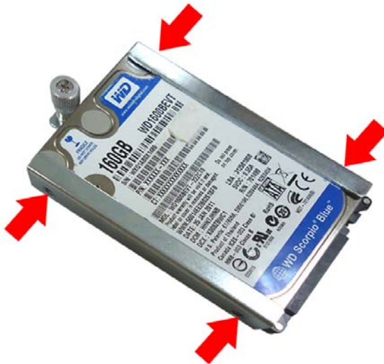
Figure 3-4: Securing the HDD
