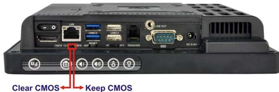
Figure 4-7: Clear CMOS Switch Location
