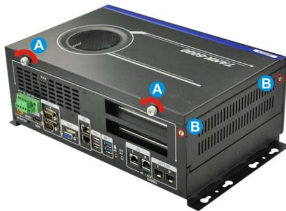
Figure 3-7: Unscrew the cover
