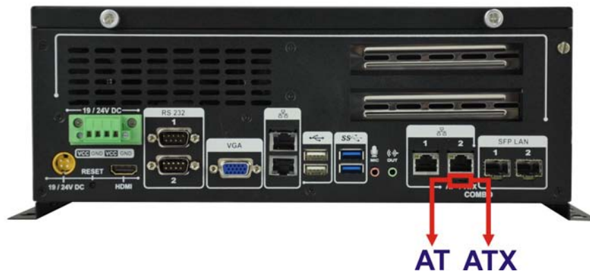
Figure 3-10: AT/ATX Switch Location
