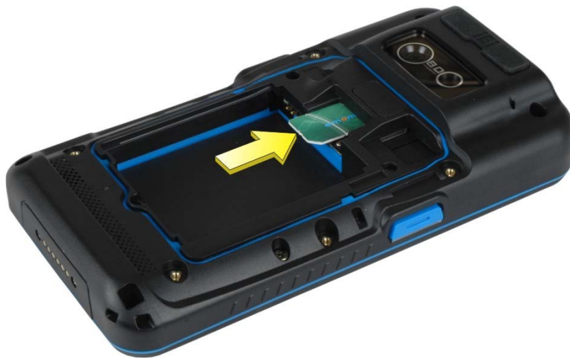
Figure 3-6: SIM Card Installation
