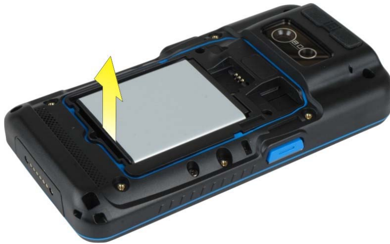
Figure 3-5: Removing the Battery
