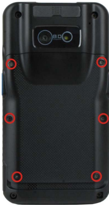
Figure 3-4: Battery Cover Retention Screws
