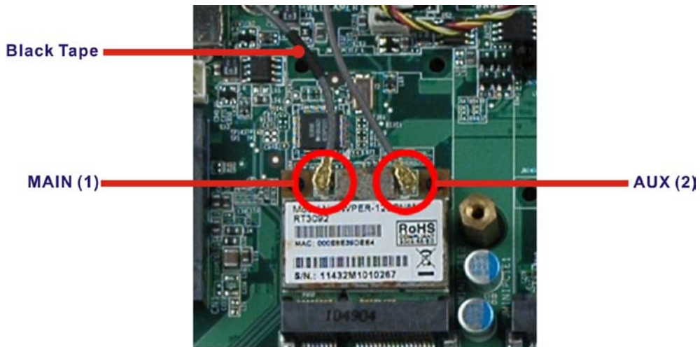
Figure 7-8: Attaching the Antennas
