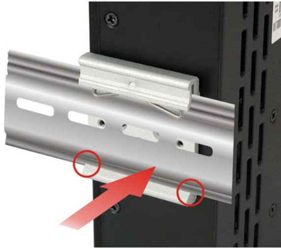
Figure 3-15: Mounting the DIN Rail
